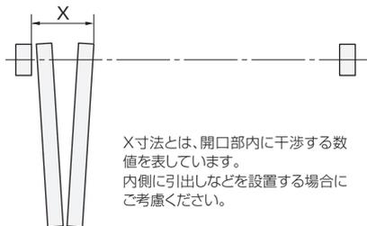
$X = 17\text{mm} + \text{戸厚} \times 2 + \text{吊元側すきま寸法}$
